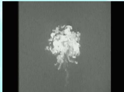
Experimental conditions: jet velocity 5cm/s discharging
