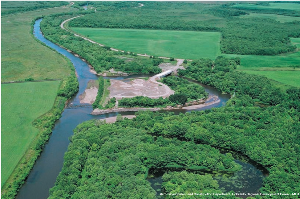
Trial to restore the meander by using the old river (Shibetsu River, Japan)
